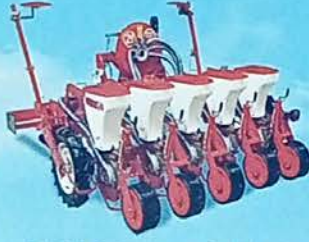
Baltalı Tip Pnömatik Hassas Ekim Makinesi Pneumatic Precision Seeder With Axe Typs
